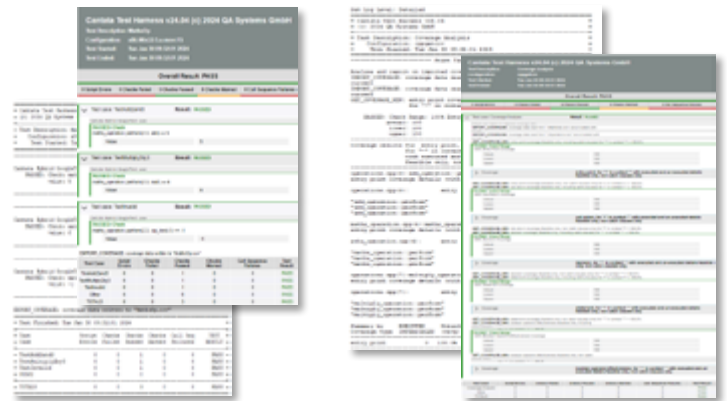
Certified Cantata Test Results for each GTest® - including aggregate code coverage achieved in both ASCII and HTML formats
